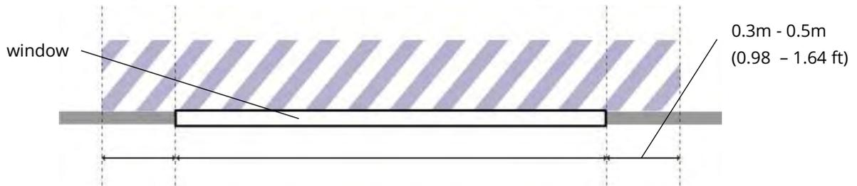
Figure 19: Clearance either side of a window
