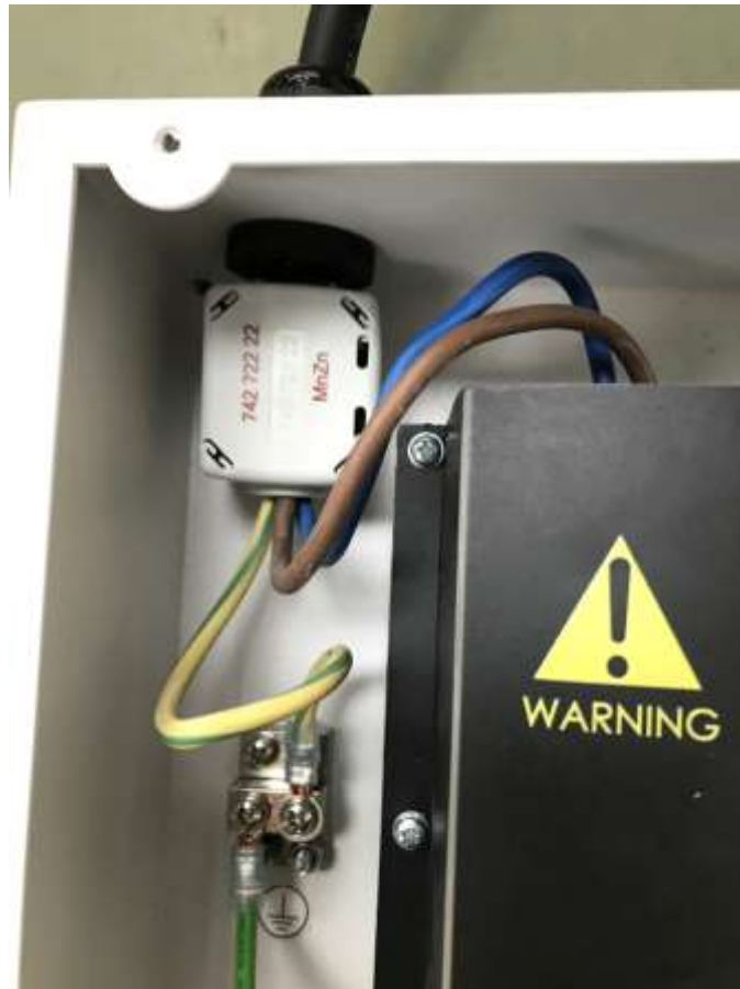
Figure 34: Ferrite installed to AC power cable
