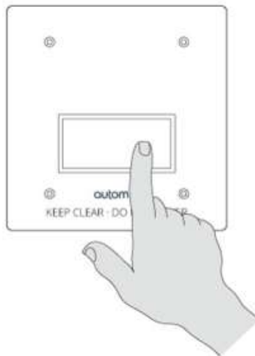
Figure 46: Gently press the outside surface of the spray head with your finger to address it
