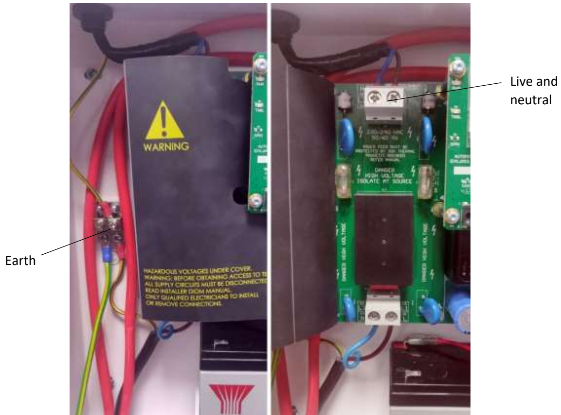
Figure 33: Black plastic PCB high voltage cover tucked closed (left) or open (right)
