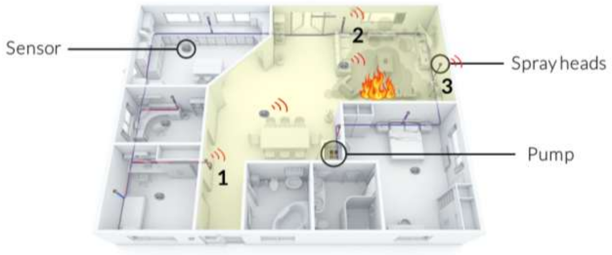
Figure 41: Yellow zone (above) contains 3 wall mounted spray heads and 2 ceiling mounted smoke sensors
