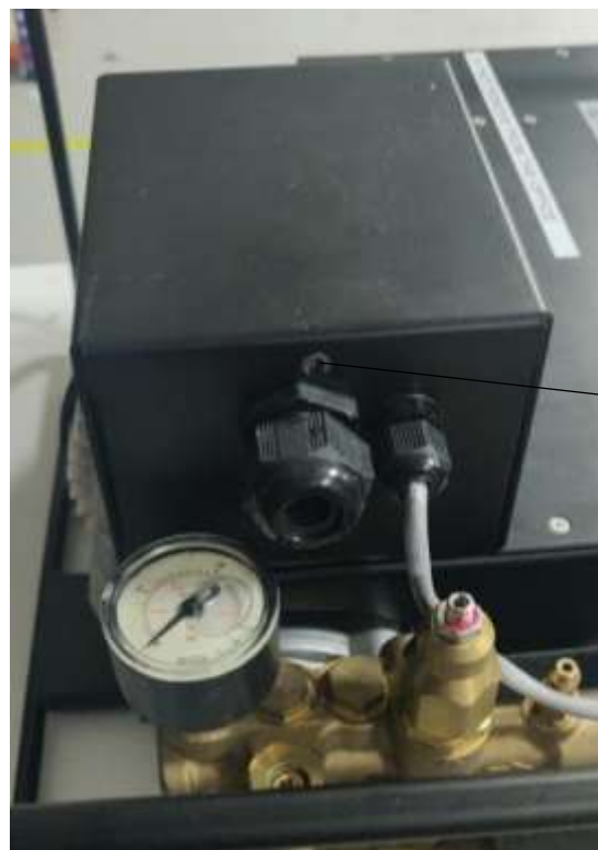
Figure 37: How to open the pump connection point
