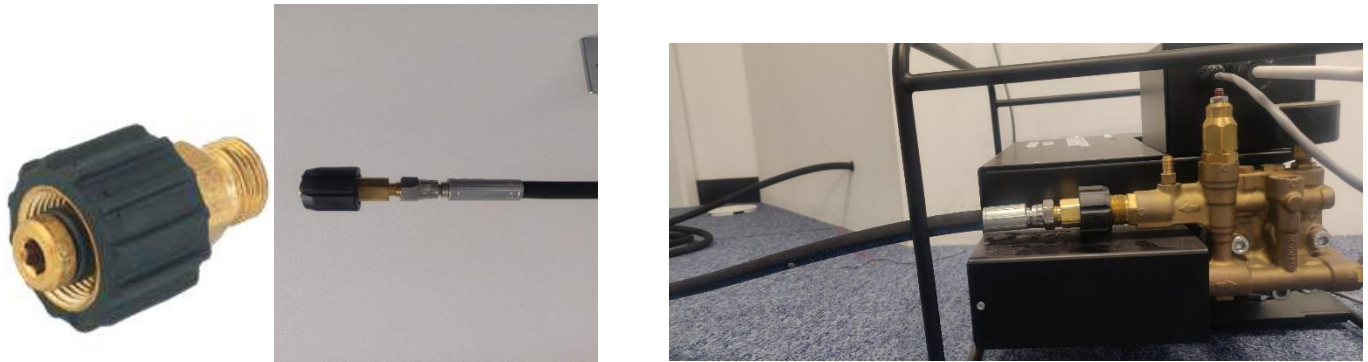
Figure 4 Connecting the high pressure hose to the pump
