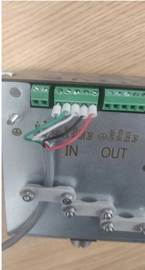
Figure 15 Correctly wired spray head terminals
