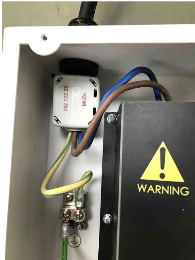
Figure 34: Ferrite installed to AC power cable
